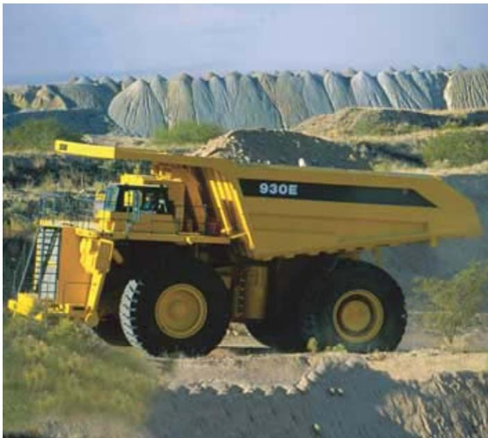
*Komatsu's 930E is a 2,000 kW truck. A 16-cylinder diesel engine drives a generator that powers electric motors on the wheels.*
