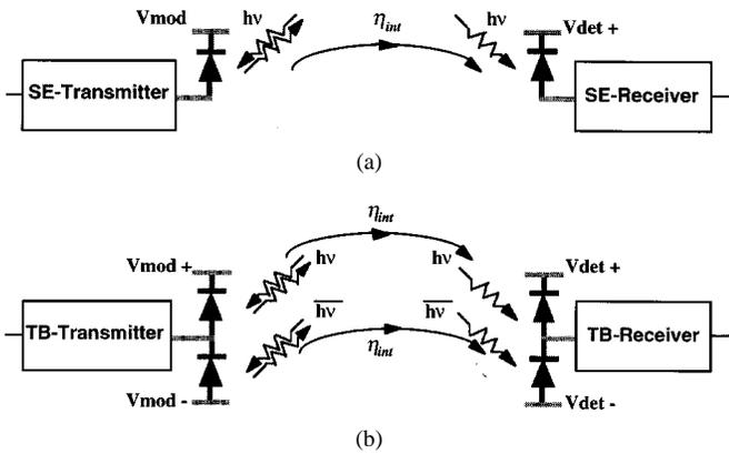
Fig. 8. Schematic of (a) single-ended (SE) optical interconnection link, (b) two-beam (TB) optical interconnection link;  $V_{det}$  and  $V_{mod}$  are the detector and transmitter bias voltages, respectively.  $\eta_{int}$  is the product of the optical system power efficiency and the modulator power efficiency.
