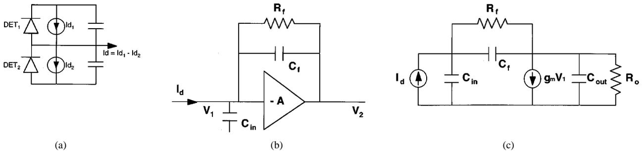
Fig. 10. (a) Differential input diode pair and (b) equivalent circuit for a typical transimpedance receiver. The feedback resistor  $R_f$ , is a PMOS inverter with a tunable gate voltage. Alternatively, the feedback element can be a parallel combination of PMOS and NMOS devices [19]. (c) Small-signal equivalent circuit for the transimpedance amplifier.
