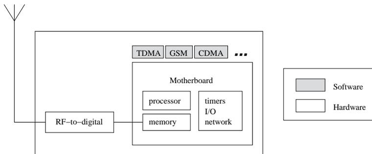
Figure 3: The Vanu Software Radio architecture
