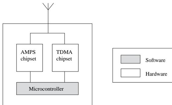
Figure 1: An example dual mode cellular handset architecture
