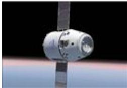
The pressurized Dragon spacecraft, developed by SpaceX, employs a flexible cargo and crew configuration, and is able to accommodate up to seven crew members per flight. Unpressurized cargo can be transported in the “trunk,” which is designed to support the pressurized capsule during ascent and contains a truss structure to hold cargo. Source: SpaceX
