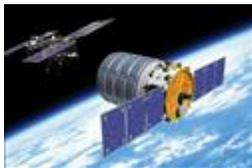
Orbital Sciences Corp. (Dulles, Va.) is leveraging its previous space vehicle experience to build an unmanned space freighter called the Cygnus. After launch into LEO atop the Taurus II rocket (below), Cygnus will maneuver to and dock with the International Space Station. Source: Orbital Sciences
