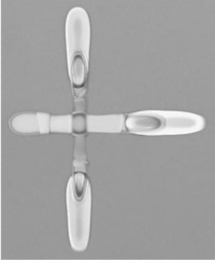
**Printing processors:** Printed transistors such as this one could bring microchips to everyday objects. Different inks are used for various parts of the transistor, which include the electrical contacts, the source and drain (top and bottom), and the controlling gate.
