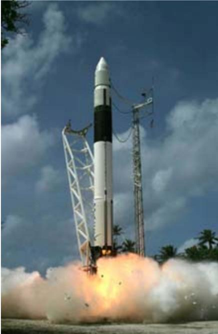
SpaceX's Falcon 1 rocket undergoes a "hot fire" or static engine test in the Kwajalein Islands in February. (Courtesy of SpaceX.)
