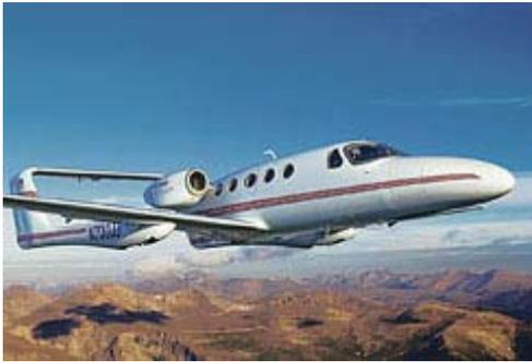
The jet is made out of composite material -- super-strong carbon-fiber plastic, which is the same material Cirrus uses in its planes and Boeing will use in its new 787 wide-body jet. Composites can be stronger than aluminum and is easier to shape into aerodynamic curves, with no rivets to disrupt airflow. That makes it cleaner through the air, and faster.
