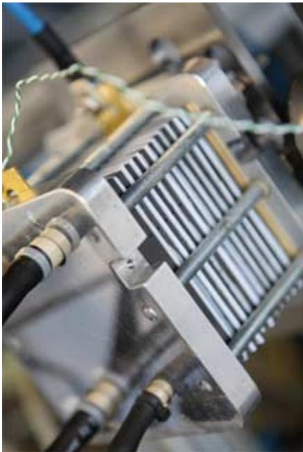
**Liquid design:** Inside ACAL Energy's fuel-cell stacks, the cathode is replaced with a platinum-free catalyst solution, which could reduce costs by 40 percent.
