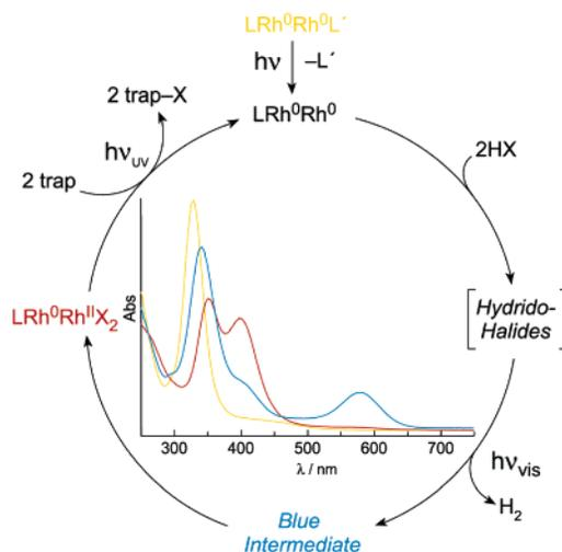
**Figure 3.** Photocycle for H<sub>2</sub> production from homogeneous HX solutions with a two-electron mixed-valence Rh<sub>2</sub><sup>0,II</sup> core as the key intermediate for Rh–X photoactivation. Only the formal oxidation states of the dirhodium core are shown; the bimetallic center is strapped by three dfpma ligands.
