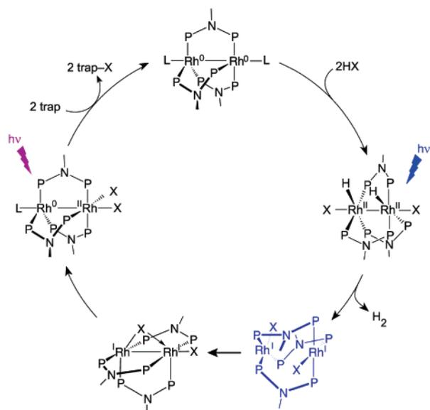
**Figure 6.** Complete photocycle for  $\text{H}_2$  generation by the dirhodium dfpma photocatalyst. Identification of the intermediates in the cycle is based on the chemistry of dirhodium and diiridium tfepma and tfepm synthetic analogues.
