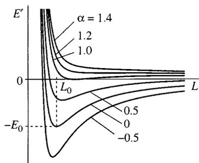
Fig. 9. Energy of a sparse array of 3-D coherently strained islands per unit surface area as a function of island size. The parameter  $\alpha$  is the ratio between the change in the surface energy upon island formation and the contribution from island edges to the elastic relaxation energy. When  $\alpha > 1$ , the system tends thermodynamically toward island coalescence. When  $\alpha < 1$ , there exists an optimal island size and the system of islands is stable against coalescence.
