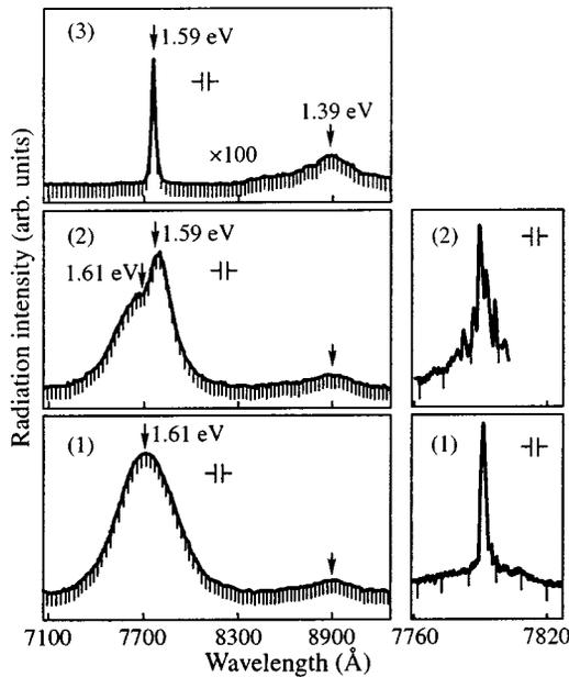
Fig. 2. Emission spectrum of the first low-threshold  $\text{Al}_x\text{Ga}_{1-x}$  DHS laser operating at room temperature (300 K),  $J_{\text{th}} = 4300 \text{ A/cm}^2$ . The current rises from 1) 0.7 A to 2) 8.3 A, and then to 3) 13.6 A.
