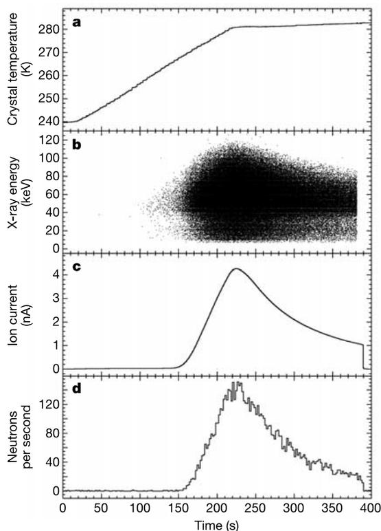
**Figure 2** Data from a single run (see also Supplementary Movie 1). **a**, Crystal temperature. The heating rate was  $12.4 \text{ K min}^{-1}$ , corresponding to a pyroelectric current of 22 nA and a heating power of 2 W. **b**, X-rays detected. **c**, Faraday cup current. **d**, Neutrons detected.
