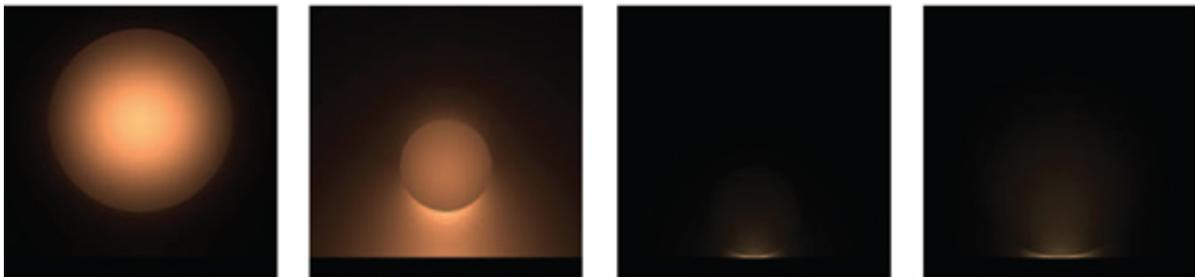
**Shape shifting:** Light is confined to different parts of the waveguide when the diameter or height of the nanowire changes. From left to right: light travels inside a 400-nanometer nanowire placed 100 nanometers above the surface; some light begins to travel between the nanowire and the surface when the diameter is reduced to 200 nanometers; when the nanowire is just two nanometers above the surface, light is trapped in the tiny gap for both 200-nanometer and 400-nanometer nanowires.
