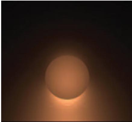
**Guiding light:** Light can be compressed between a semiconductor nanowire and a smooth sheet of silver, depending on the nanowire's diameter and its height above the metal surface. Here, light is confined in a 100-nanometer gap by a nanowire with a 200-nanometer diameter. Credit: Rupert Oulton, UC Berkeley
