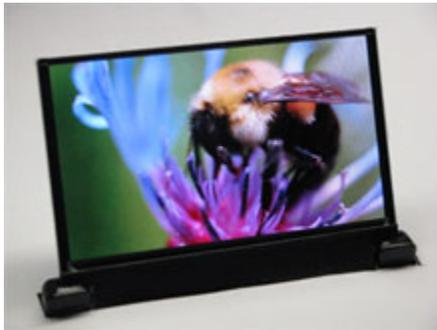
**Longer life:** DuPont has developed longer-lasting OLED materials that can be printed using cheap, simple techniques to make displays like this one.
