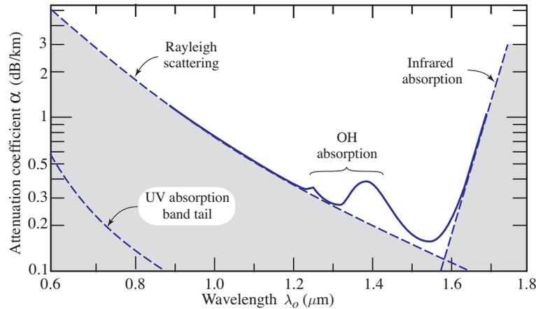
**Figure 9.3-2** Attenuation coefficient  $\alpha$  of silica glass versus wavelength  $\lambda_o$ . There is a local minimum at  $1.3 \mu\text{m}$  ( $\alpha \approx 0.3 \text{ dB/km}$ ) and an absolute minimum at  $1.55 \mu\text{m}$  ( $\alpha \approx 0.15 \text{ dB/km}$ ).
