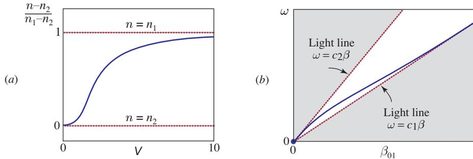
**Figure 9.2-8** Schematic illustrations of the propagation characteristics of the fundamental  $LP_{01}$  mode. (a) Effective refractive index  $n = \beta/k_o$  as a function of the  $V$  parameter. (b) Dispersion relation ( $\omega$  versus  $\beta_{01}$ ).
