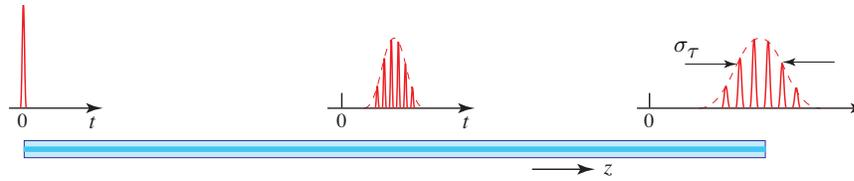
**Figure 9.3-4** Pulse spreading caused by modal dispersion.
