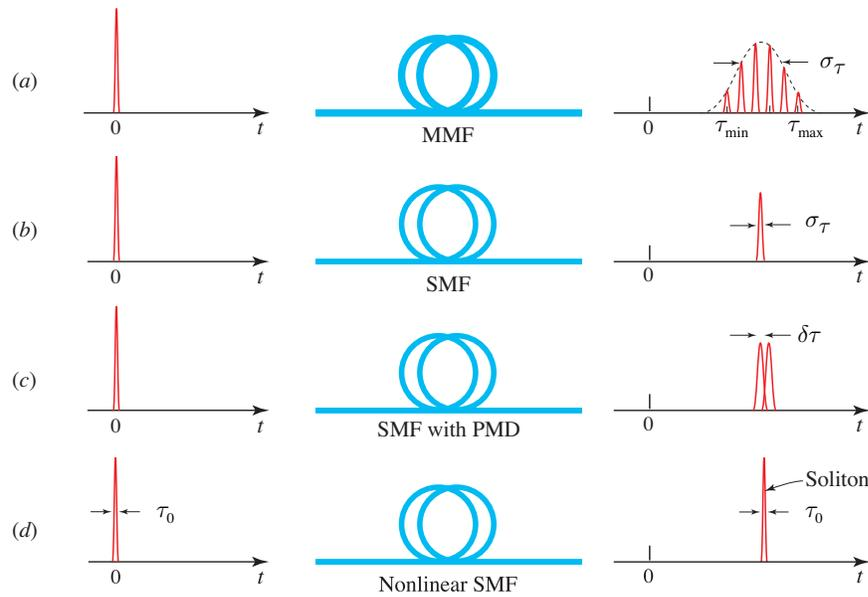
**Figure 9.3-9** Broadening of a short optical pulse after transmission through different types of fibers. (a) Modal dispersion in a multimode fiber (MMF). (b) Material and waveguide dispersion in a single-mode fiber (SMF). (c) Polarization mode dispersion (PMD) in a SMF. (d) Soliton transmission in a nonlinear SMF.
