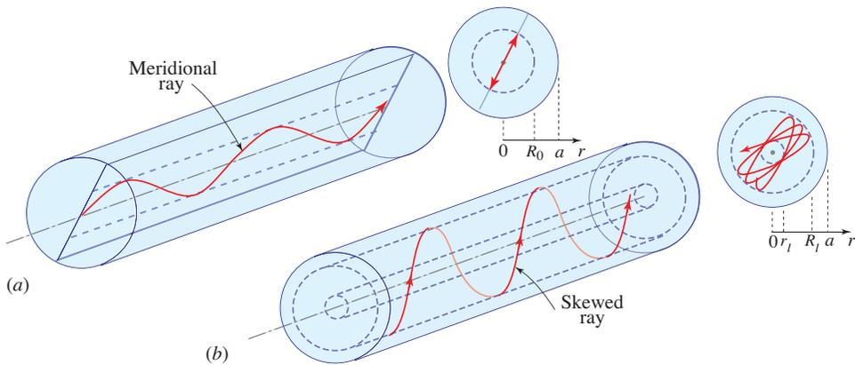
**Figure 9.1-6** Guided rays in the core of a GRIN fiber. (a) A meridional ray confined to a meridional plane inside a cylinder of radius  $R_0$ . (b) A skewed ray follows a helical trajectory confined within two cylindrical shells of radii  $r_1$  and  $R_1$ .
