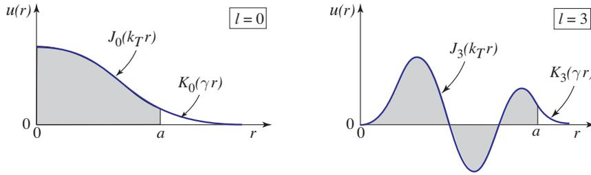
**Figure 9.2-2** Examples of the radial distribution  $u(r)$  provided in (9.2-6) for  $l = 0$  and  $l = 3$ . The shaded and unshaded areas represent the fiber core and cladding, respectively. The parameters  $k_T$  and  $\gamma$ , and the two proportionality constants in (9.2-6), have been selected such that  $u(r)$  is continuous and has a continuous derivative at  $r = a$ . Larger values of  $k_T$  and  $\gamma$  lead to a greater number of oscillations in  $u(r)$ .
