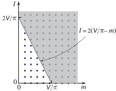
**Figure 9.2-6** The indexes of guided modes extend from  $m = 1$  to  $m \approx V/\pi - l/2$  and from  $l = 0$  to  $l \approx 2V/\pi$ , as displayed by the unshaded area.
