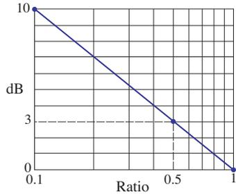
**Figure 9.3-1** The dB value of a ratio. For example, 3 dB is equivalent to a ratio of 0.5; 10 dB corresponds to  $\mathcal{T} = 0.1$ ; and 20 dB corresponds to  $\mathcal{T} = 0.01$ .
