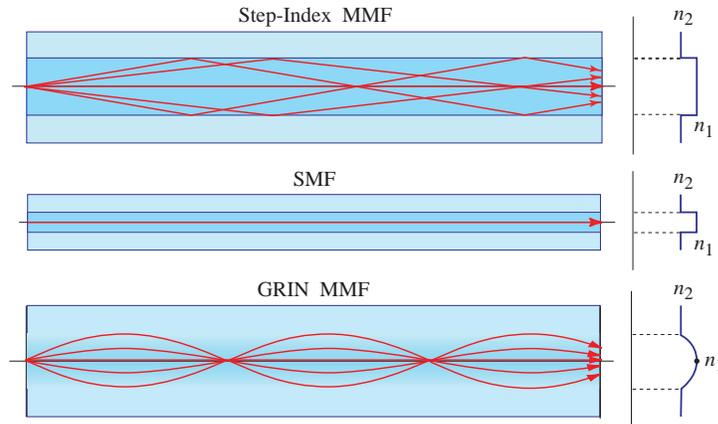
**Figure 9.0-2** Geometry, refractive-index profile, and typical rays in a step-index multimode fiber (MMF), a single-mode fiber (SMF), and a graded-index multimode fiber (GRIN MMF).
