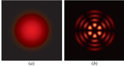
**Figure 9.2-4** Intensity distributions of (a) the  $LP_{01}$  and (b) the  $LP_{34}$  modes in the transverse plane, assuming an azimuthal dependence of the form  $\cos l\phi$ . The distribution of the fundamental  $LP_{01}$  mode is similar to that of the Gaussian beam discussed in Chapter 3.
