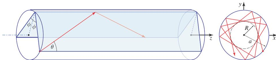
**Figure 9.1-2** A skewed ray lies in a plane offset from the fiber axis by a distance  $R$ . The ray is identified by the angles  $\theta$  and  $\phi$ . It follows a helical trajectory confined within a cylindrical shell with inner and outer radii  $R$  and  $a$ , respectively. The projection of the ray on the transverse plane is a regular polygon that is not necessarily closed.
