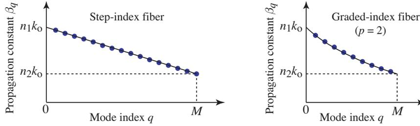
**Figure 9.2-13** Dependence of the propagation constants  $\beta_q$  on the mode index  $q = 1, 2, \dots, M$  for a step-index fiber ( $p \rightarrow \infty$ ) and for an optimal graded-index fiber ( $p = 2$ ).
