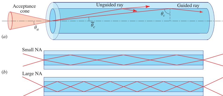
**Figure 9.1-3** (a) The acceptance angle  $\theta_a$  of a fiber. Rays within the acceptance cone are guided by total internal reflection. The numerical aperture  $\text{NA} = \sin \theta_a$ . The angles  $\theta_a$  and  $\bar{\theta}_c$  are typically quite small; they are exaggerated here for clarity. (b) The light-gathering capacity of a large NA fiber is greater than that of a small NA fiber.
