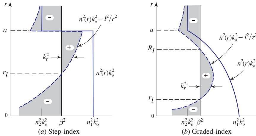
**Figure 9.2-11** Dependence of  $n^2(r)k_o^2$ ,  $n^2(r)k_o^2 - l^2/r^2$ , and  $k_r^2 = n^2(r)k_o^2 - l^2/r^2 - \beta^2$  on the position  $r$ . At any  $r$ ,  $k_r^2$  is the width of the shaded area with the + and - signs denoting positive and negative values of  $k_r^2$ , respectively. (a) Step-index fiber:  $k_r^2$  is positive in the region  $r_l < r < a$ . (b) Graded-index fiber:  $k_r^2$  is positive in the region  $r_l < r < R_l$ .
