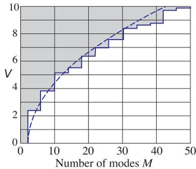
**Figure 9.2-5** Total number of modes  $M$  versus the fiber parameter  $V = 2\pi(a/\lambda_o)\text{NA}$ . Included in the count are the two helical polarities for each mode with  $l > 0$  and the two polarizations per mode. For  $V < 2.405$ , there is only a single mode, the fundamental  $\text{LP}_{01}$  mode with two polarizations. The dashed curve is the relation  $M = 4V^2/\pi^2 + 2$ , which provides an approximate formula for the number of modes when  $V \gg 1$ .
