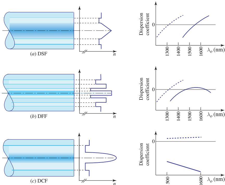
**Figure 9.3-6** Refractive-index profiles with schematic wavelength dependences of the material dispersion coefficient (dashed curves) and the combined material and waveguide dispersion coefficients (solid curves) for (a) dispersion-shifted fiber (DSF), (b) dispersion-flattened fiber (DFF), and (c) dispersion-compensating fiber (DCF).
