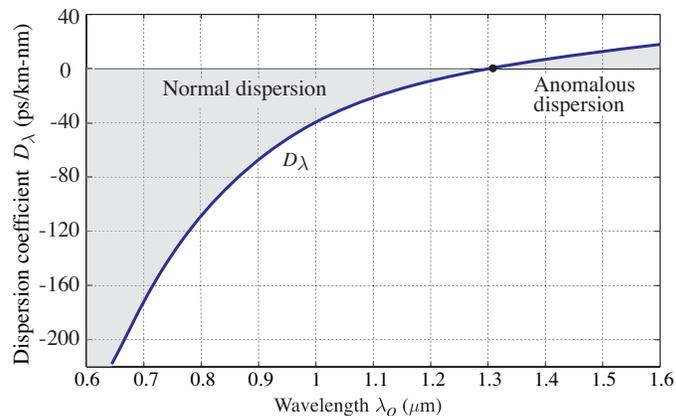
**Figure 9.3-5** Dispersion coefficient  $D_\lambda$  for a silica-glass fiber as a function of wavelength  $\lambda_o$ . The result is similar to, but distinct from, that of fused silica (see Fig. 5.6-5).
