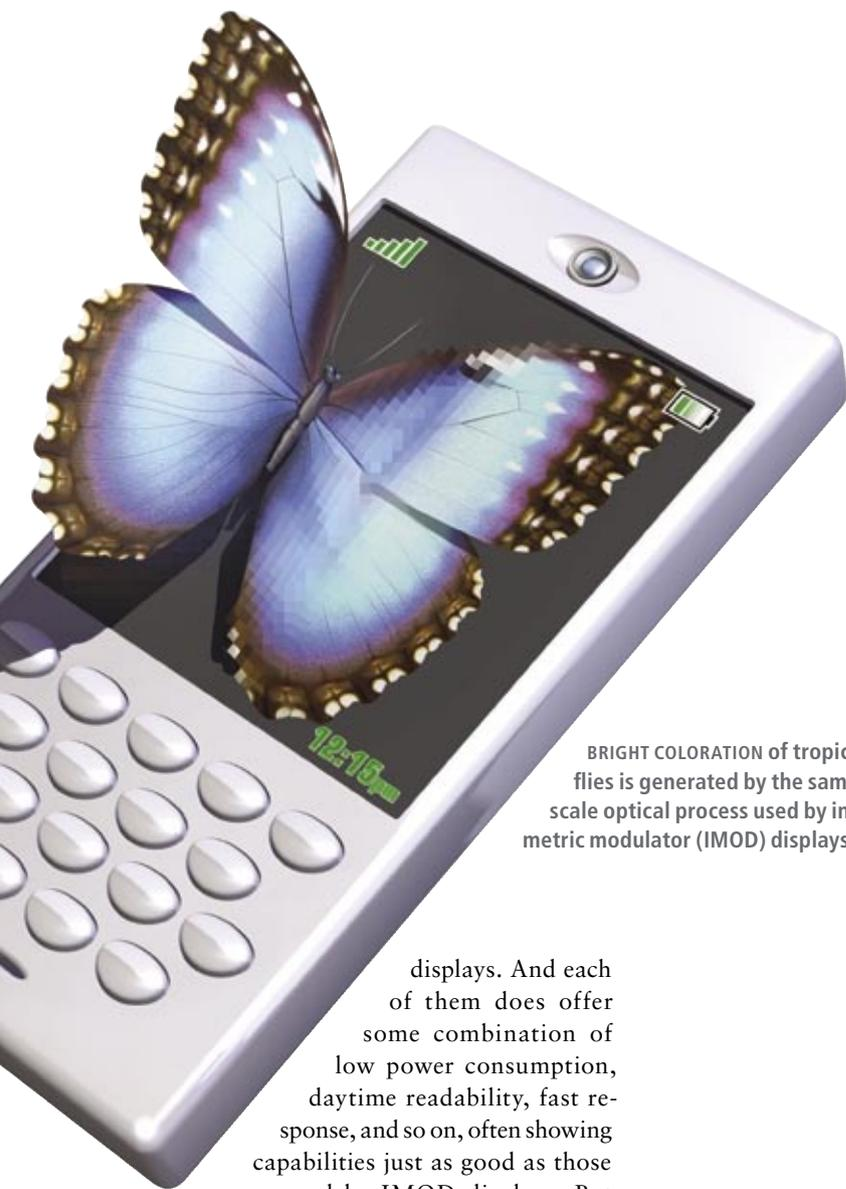
BRIGHT COLORATION of tropical butterflies is generated by the same nanoscale optical process used by interferometric modulator (IMOD) displays.
