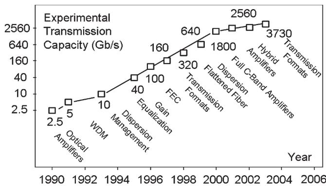
Fig. 4. Capacity of transoceanic-length transmission experiments measured in Gb/s, and the associated technology milestones. During the 1990s, the demonstrated capacity rapidly increased as more and more optical bandwidth was used. The rate of increase slowed dramatically in the early 2000s when the full EDFA bandwidth was exploited.
