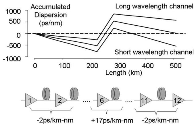
Fig. 15. Accumulated dispersion versus distance for the amplifier chain displayed in the bottom of the figure. The majority of the fiber in this dispersion map has an average dispersion of  $-2 \text{ ps/km} \cdot \text{nm}$ . This negative dispersion is compensated by using a conventional single-mode fiber that has an average dispersion of about  $+17 \text{ ps/km} \cdot \text{nm}$ .
