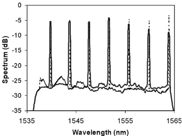
Fig. 12. Measured and simulated optical spectra for seven WDM signals uniformly spread across the passband of a 6650-km amplifier chain [22]. Note that the optical powers and SNRs for each channel are similar.
