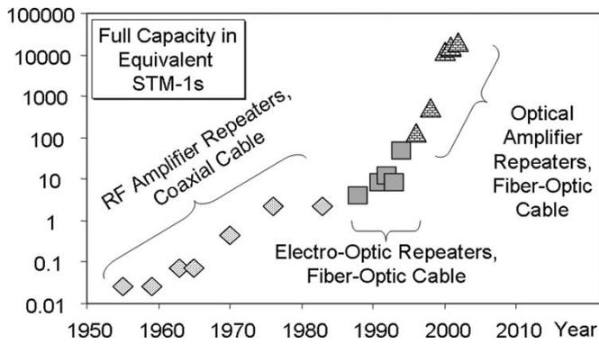
Fig. 3. Full capacity of transatlantic cable systems installed over the past five decades, displayed in STM-1's (or "equivalent STM-1's" for the analog systems).
