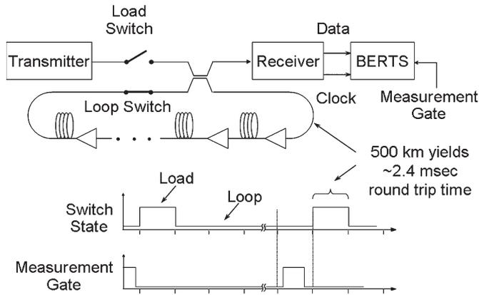
Fig. 25. Top: Block diagram for a circulating-loop experiment. Bottom: Timing diagram for a circulating-loop measurement showing the optical switch states and the time gate for making measurements.
