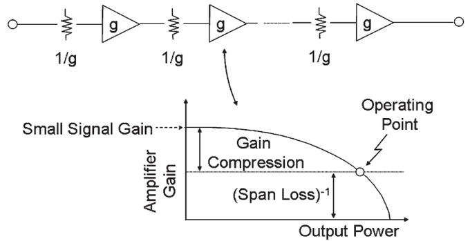
Fig. 7. Gain compression in the EDFA is used for power control on the amplifier chain. The small signal gain of each EDFA is designed to be larger than is needed to compensate the loss of the fiber span. This creates a stable operating point where EDFA gain equals the span's attenuation.
