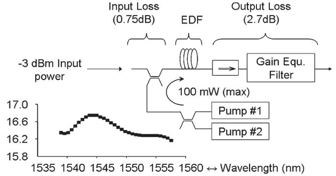
Fig. 27. Block diagram for an EDFA with redundant pump lasers. The average input attenuation is 0.75 dB and the average output attenuation is 2.7 dB. The curve at the bottom left shows the calculated gain assuming a flat output power and an average input power of  $-3$  dBm.
