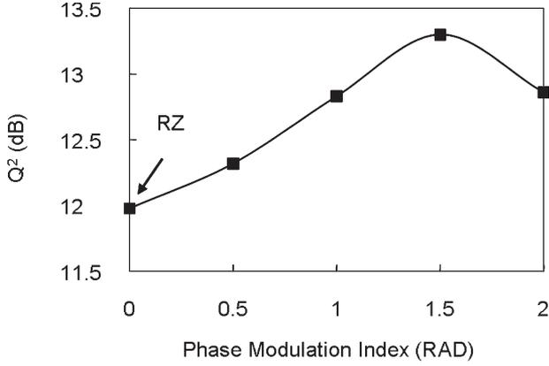
Fig. 21.  $Q$ -factor versus phase-modulation index for channel 2 [38] at 7900 km, employing CRZ.
