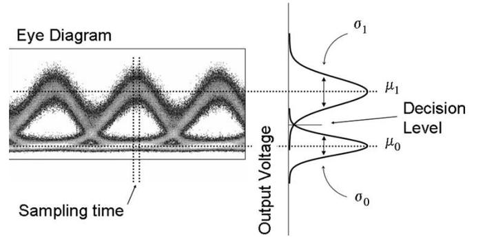
Fig. 22. Typical RZ eye diagram at the input to a decision circuit. The voltage samples that fall within the sampling window are used to form the histogram on the right-hand side. The upper and lower lobes of the voltage histogram have an associated mean and standard deviation.
