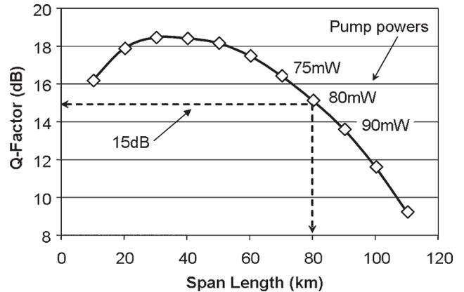
Fig. 28. Calculated  $Q$ -factor versus span length using (2), (3), and (11), and the values in Table I. These data were calculated for a fixed path-averaged power of  $124 \mu\text{W}$  per channel.
