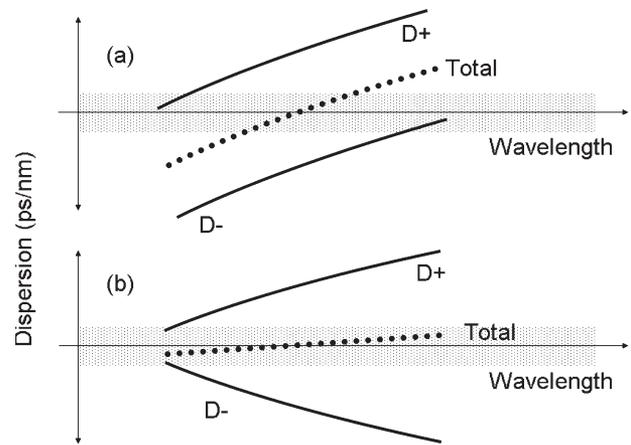
Fig. 16. Dispersion versus wavelength for (a) a conventional dispersion map and (b) a dispersion map using dispersion-flattened fiber.
