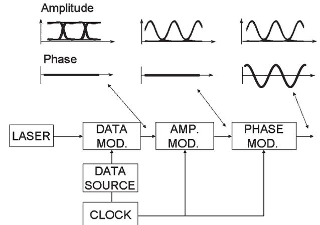
Fig. 19. Block diagram of a CRZ transmitter. Also shown are typical waveforms for the intensity and phase of the optical signal at intermediate points within the transmitter.
