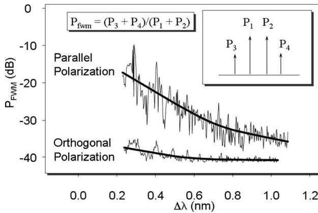
Fig. 18. Measured FWM efficiency versus channel separation in a 500-km amplifier chain. The upper wavelength channel is placed at the system's zero-dispersion wavelength. The upper curve is for parallel-polarization launch, and the lower line is for orthogonal-polarization launch.
