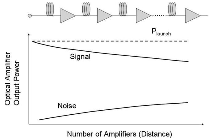
Fig. 8. Signal and noise propagation along a chain of optical amplifiers. The average signal level decreases along the amplifier chain since the noise generated in each amplifier accumulates, and the total output power of each amplifier is fixed by gain compression.
