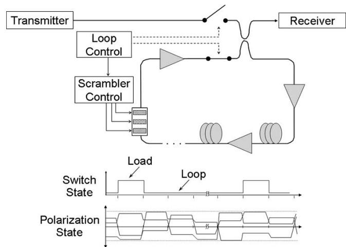
Fig. 26. Top: Block diagram of a circulating-loop experiment with a loop-synchronous polarization switching (modeled after [49]). Bottom: Simple timing diagram for the loop experiment along with typical drive signals for the polarization controller.
