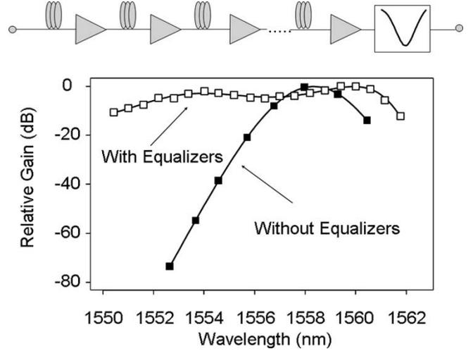
Fig. 10. Relative gain versus wavelength in a 6300-km amplifier chain. The optical bandwidth was expanded by about  $3\times$  using passive gain-equalizing filters.
