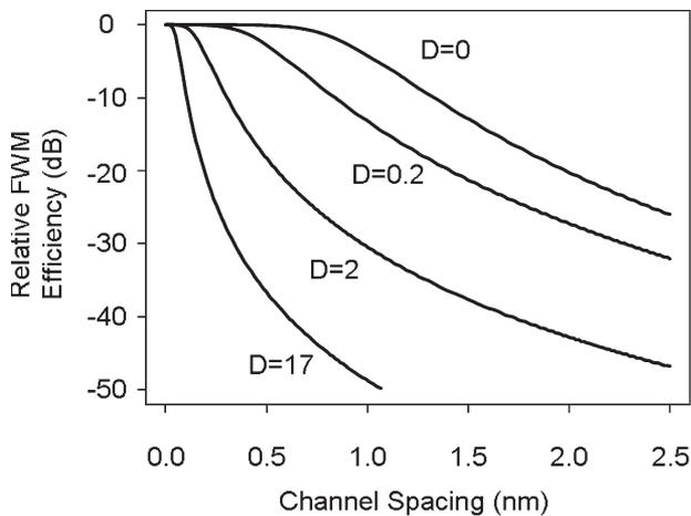
Fig. 14. Nonlinear mixing efficiency versus channel separation for two optical channels propagating through a single-mode optical fiber. The calculation is performed for four different values of chromatic dispersion. The vertical axis was arbitrarily set to 0 for small channel spacing (following the model in [24]).
