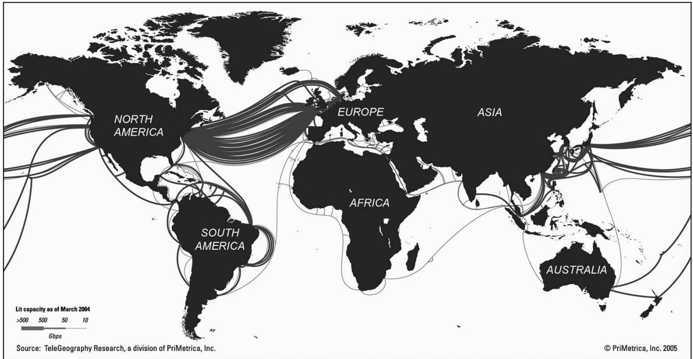
Fig. 1. World map showing the major undersea-cable systems that are in operation today. The thickness of the cable paths indicates the “Lit” capacity on each route. Source: TeleGeography Research, a division of PriMetrica, Inc.
