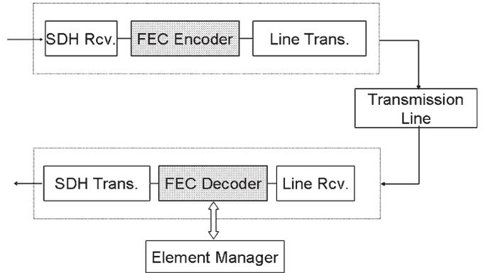
Fig. 23. FEC encoder and decoder are located between the client-side and line-side transponders. The actual bit rate transmitted on the line side is increased by the FEC overhead, which is typically between 7–25% for optical transmission systems.
