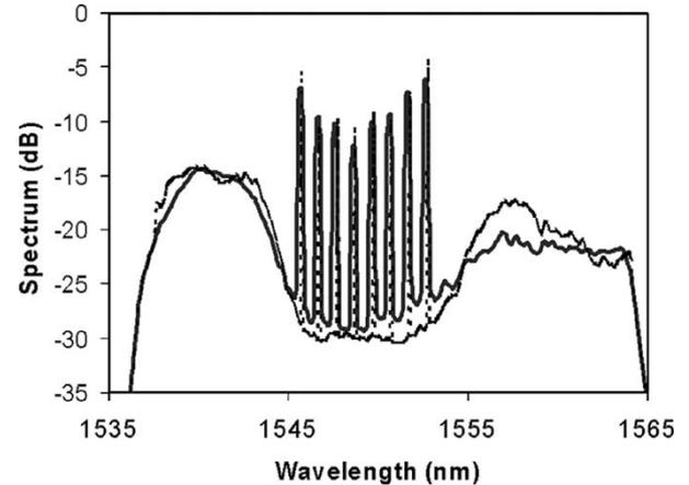
Fig. 13. Similar plot to that of Fig. 12 for the measured and simulated optical spectra of eight WDM channels after passing through a 6650-km-length system. In this case, the eight WDM channels were concentrated in the center of the passband. Note that the tightly spaced channels have depressed the gain for the center channel [22].
