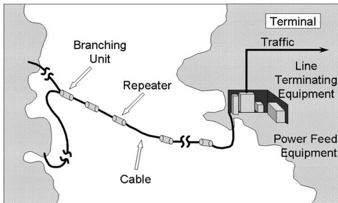
Fig. 2. High-level view of an undersea-cable communications system. The undersea portion contains cables and repeaters. The land portion contains equipment to power the undersea cable, undersea network-management equipment, and line-terminating equipment to convert the terrestrial-grade signal to a format that can go through the long undersea cable.
