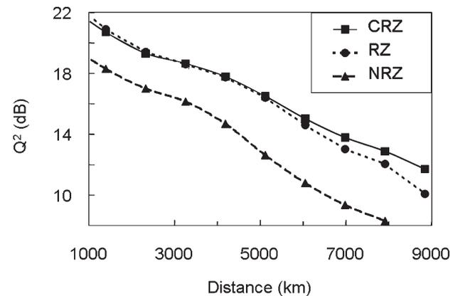
Fig. 20.  $Q$ -factor versus transmission distance for edge channel 2 of [38] with different modulation formats (CRZ with 1 rad phase modulation).
