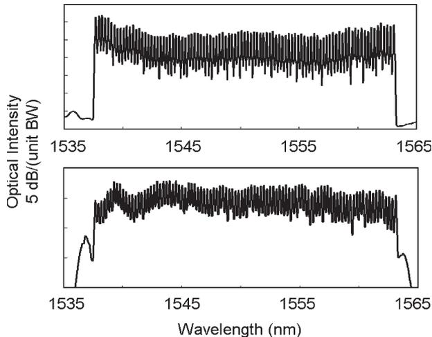
Fig. 11. Optical spectra from a field trial using  $96 \times 12.3$  Gb/s per fiber over the first installed dispersion-flattened transpacific system, 9000-km long, part of the TGN. (Top) Input spectrum in Oregon, USA, and (bottom) output spectrum after the 9000-km transmission in Toyohashi, Japan, for the 96 channels at 12.3 Gb/s [12].
