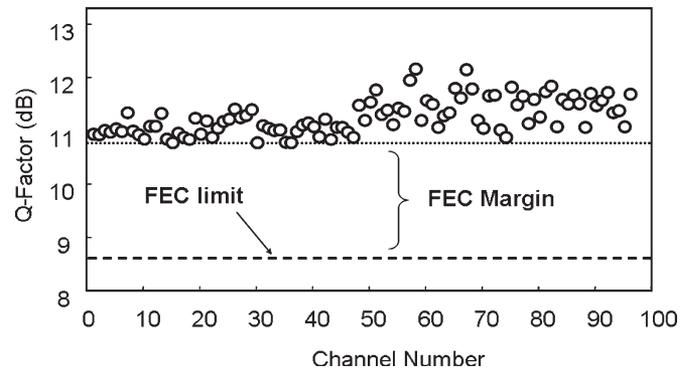
Fig. 6. Measured  $Q$ -factor versus channel number after the 9000-km transmission for the 96-channel operation on the TGN Pacific system. The lower dashed horizontal line labeled "FEC limit" is the  $Q$ -factor corresponding to error-free operation [12].
