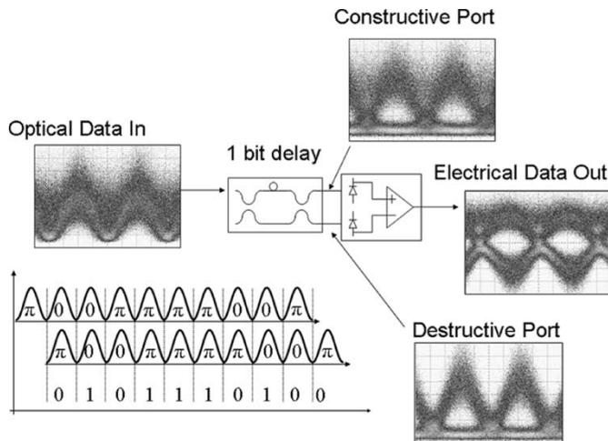
Fig. 29. Block diagram of a DPSK receiver, along with typical eye diagrams at intermediate points within the receiver. The eye diagrams were measured after 11 000 km [58].
