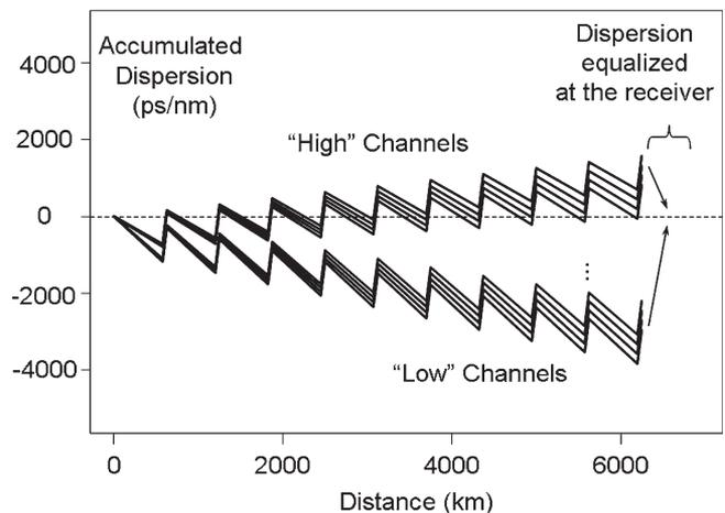
Fig. 17. Accumulated dispersion over an entire 6000-km transmission system that uses conventional non-slope-matched fibers.
