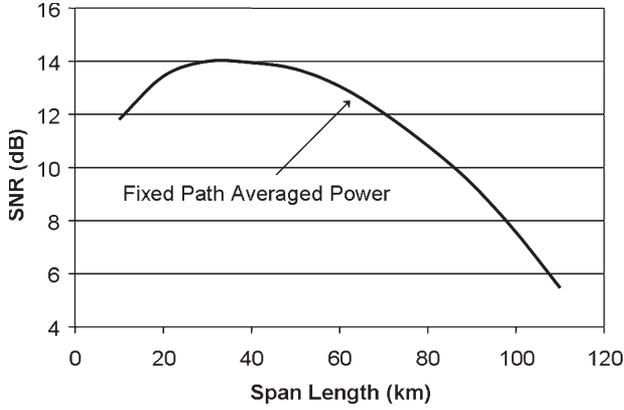
Fig. 9. Calculation of received SNR versus span length using (2) and (3). The input parameters are given in Table I. The calculation is performed for a fixed path-averaged power of  $124 \mu\text{W}$ . This simplification ignores the signal decay shown in Fig. 8.
