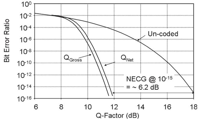
Fig. 24. Output BER versus input  $Q$ -factor. The top curve labeled “uncoded” is simply (7) or (8) plotted for input  $Q$ -factor expressed in decibels. The curve labeled  $Q_{\text{Gross}}$  gives the input/output BER characteristics for the standard G.709 7% Reed-Solomon FEC algorithm. The curve labeled  $Q_{\text{Net}}$  is shifted to the right by  $\sim 0.28$  dB, which corrects for the added 7% increase in bit rate.
