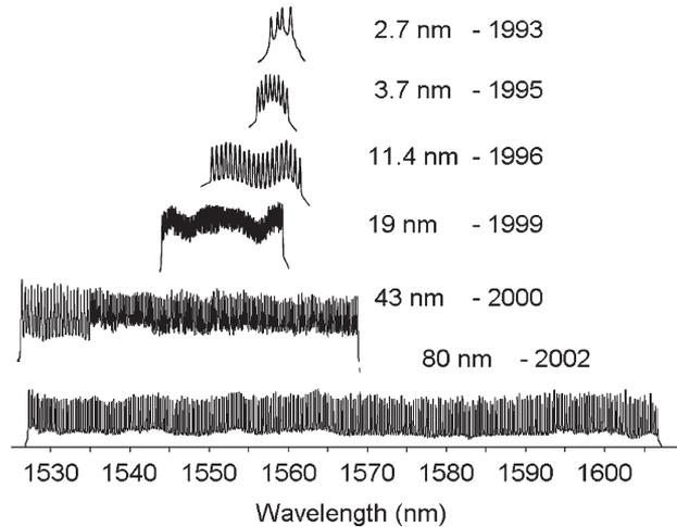
Fig. 5. Received optical spectrum of various WDM transmission experiments over the past 12 years. In each of the six curves, the amount of bandwidth is displayed along with the year that the work was published. The 43-nm result in the year 2000 corresponds to the full EDFA C-band. The 80-nm result in the year 2002 corresponds to the EDFA's C- and L-bands.
